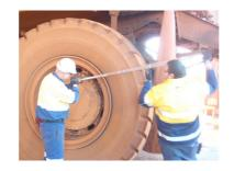
The PIG777, extension can be made to suit any Torque Wrench in the market up to 2000ft-lb, it comes complete with Pinch Guard, and tool support for the extension to be supported from a spring balancer and platform, Making this task safer & quicker.
